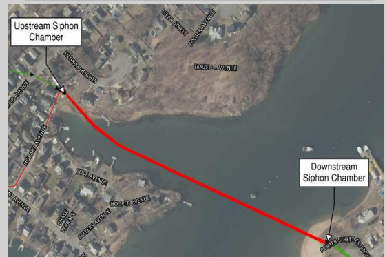
Alignment of the triple barrel Bass River Siphons
